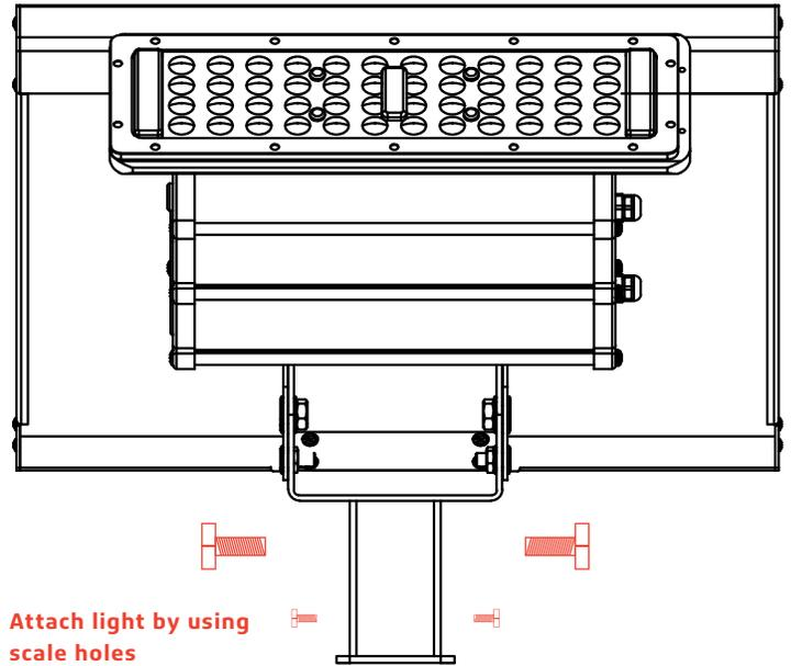
Attach light by using scale holes
