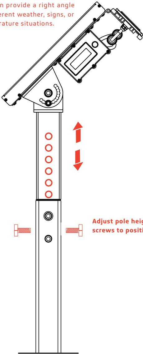
Adjust pole height, then tighten screws to position.
