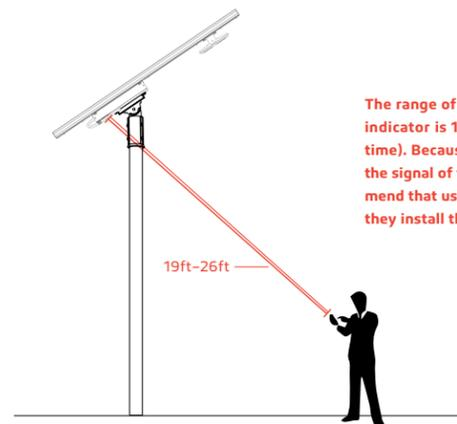
The range of the remote control to the indicator is 16ft (Day time) to 33ft (Night time). Because the sunlight will impact the signal of the remote control, we recommend that users setup the mode before they install the light.
